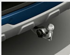
□ The electric towbar is approved for heavy loads of up to 3.5t.
