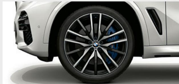
□ 22" M light alloy Double-spoke style 742 M wheels, Bicolour, front 9.5 J x 22 with 275/35 R22 tyres, rear 10.5 J x 22 with 315/30 R22 tyres. (Optional for M Sport, M50d and M50i models only).
