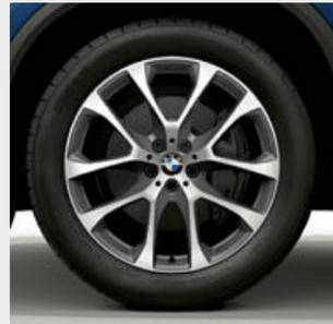
□ 20" light alloy V-spoke style 738 wheels, Bicolour, front 9 J x 20 with 275/45 R20, rear 10.5 J x 20 with 305/40 R20 run-flat tyres. (Optional for xLine models only).
