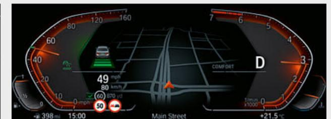
□ The automatic Speed Limit Assist adapts the Active Cruise Control dynamically to upcoming speed limits. These are determined along the probable route by the navigation system and checked by the camera. The information provided is continuously updated by the entire fleet. Featured as part of Driving Assistant Professional.
