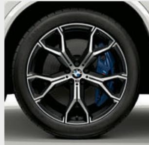
□ 21" M light alloy Y-spoke style 741 M wheels, Bicolour, front 9.5 J x 21 with 275/40 R21, rear 10.5 J x 21 with 315/35 R21 run-flat tyres. (Optional for M Sport models only).
