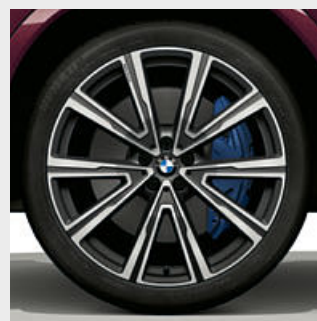
□ 22" BMW Individual light alloy V-spoke style 746 I wheels, front 9.5J x 22 with 275/35 R22, rear 10.5J x 22 with 315/30 R22 mixed tyres. Also available with the M Sport Plus Package on M Sport models.
