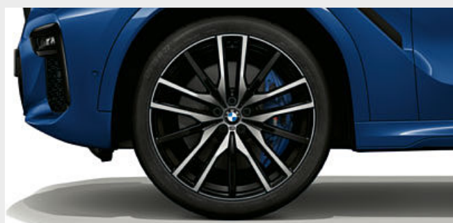
□ 22" M light alloy Double-spoke style 742 M wheels, front 9.5J x 22 with 275/35 R22 tyres, rear 10.5J x 22 with 315/30 R22 tyres. Optional for M Sport, M50i and M50d models.
