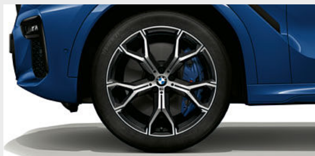
■ 21" M light alloy Y-spoke style 741 M wheels with mixed, run-flat tyres, front 9.5J x 21 with 275/40 R21 tyres, rear 10.5J x 21 with 315/35 R21 tyres. Standard on xDrive40i and xDrive30d M Sport models.
