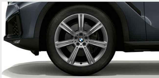
□ 20" light alloy Star-spoke style 736 wheels, front 9J x 20 with 275/45 R20, rear 10.5J x 20 with 305/40 R20 mixed, run-flat tyres. Optional on the xDrive40i and xDrive30d Sport models.
