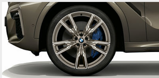
■ 22" M light alloy V-spoke style 747 M wheels, front 9.5J x 22 with 275/35 R22, rear 10.5J x 22 with 315/30 R22 mixed tyres. Standard on the M50i and M50d models.
