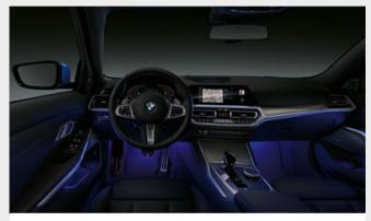
■ Ambient lighting, including Ambient contour lighting in the front and rear doors, creates a relaxed lighting atmosphere in the interior. The 11 dimmable lighting designs also include a dynamic function in four applications. The light carpet illuminates the area in front of the vehicle doors when getting in and out.
