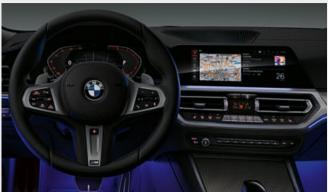
■ The BMW Live Cockpit Professional features a display cluster consisting of a fully digital 12.3" instrument display and a high-resolution 10.25" Control Display as well as the BMW Operating System 7.0. Exclusively available as standard for M Sport, M Sport Plus Edition and M340i xDrive models.
