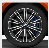
■ 18" M light alloy Doublespoke style 790 M wheels, Bicolour Orbit Grey, front 7.5 J x 18 with 225/45 R18, rear 8.5 J x 18 with 255/40 R18 run-flat tyres. Standard on M Sport models.1
